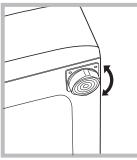
een adjusted correctly. 1. Install the washer-dryer on a flat sturdy floor, without resting it up against walls, furniture cabinets or other. 2. If the floor is not perfectly level, compensate for any unevenness by tightening or loosening the adjustable front feet (see figure); the angle of inclination, measured according to the worktop, must not exceed 2°.
